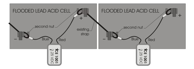
The **acutix** ICE 1001 works by bypassing any current that is not required by each cell. Approximately 50mA of extra current (over & above that required by the weakest cell) should bypass.
